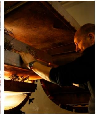
BOTTOM RIGHT | The unique copper berry chamber made in the 1920s to extract essential oils from botanicals to ensure the maximum uptake of flavor and aroma
